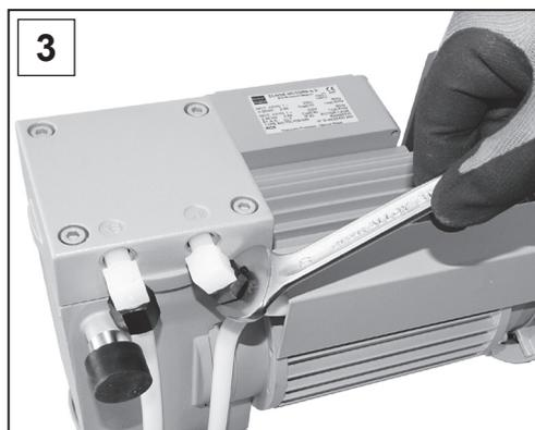
3. Tighten the union nuts at first by hand. Then tighten the union nuts one full turn using the open-ended wrench; open-ended wrench width 17 mm.
