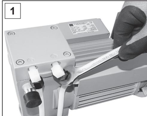
1. Loosen the union nuts at the pump heads; open-ended wrench width 17 mm.
